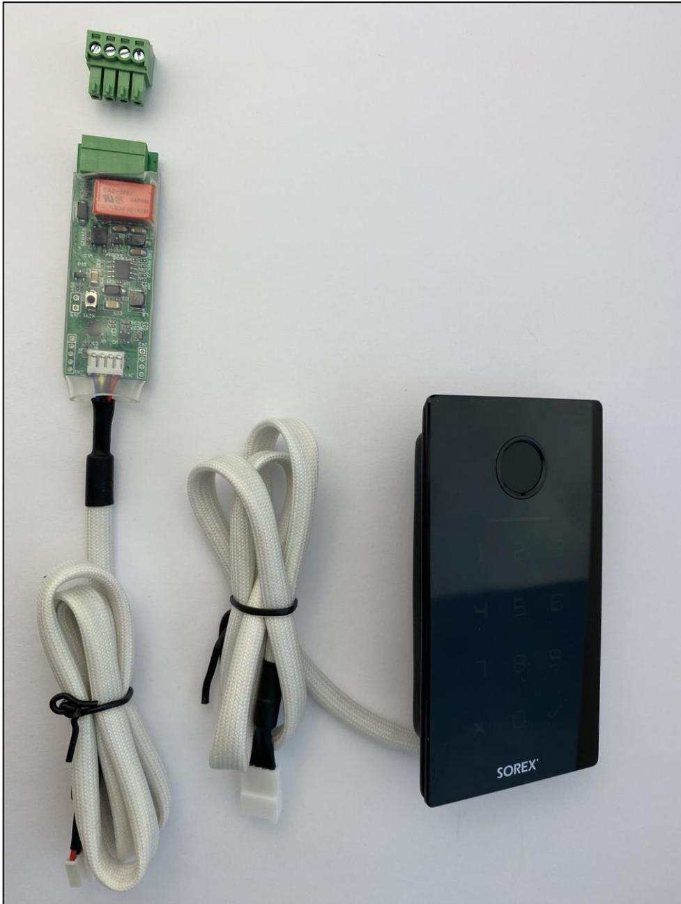
1. Unilock indoor unit incl. cable for connection with outdoor unit
